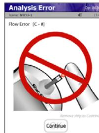
Either insufficient sample or the sample was applied incorrectly. Repeat test with a new strip.
