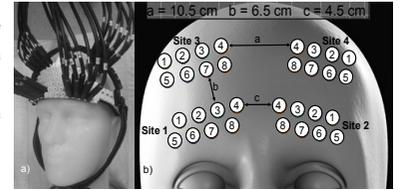
Figure 1. a) Photograph of headgear with the four-site optode array; b) Diagram of the optode arrangements in each site, and the inter-site distances.
