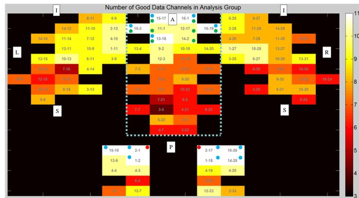
Figure 2: Topographic map displaying the number of times each data channel was marked good across the 11 analysis patients. Blue dots represent the 12 good channels across all 11 patients. Green dots represent the channels used in the 8-channel forehead array. Red dots represent the INVOS-mimic array. A = anterior, P = posterior, I = inferior, S = superior, L = left, R = right
