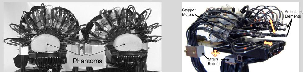
Fig. 1. Left: photograph of the sensing heads used for simultaneous dual-breast measurements, with breast-simulating phantoms in place. Right: side-view photograph of one of the left-breast sensing head.
