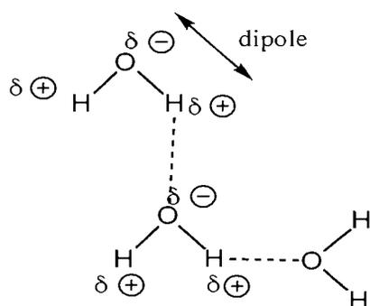
hydrogen bonding in water.
