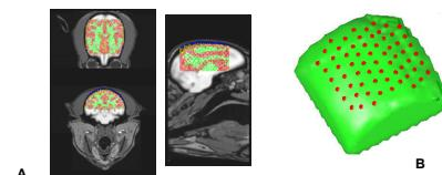
Figure 4. (A) Segmented FEM mesh of an optical imaging region; (B) An FEM model with 64 sources and 64 detectors.
