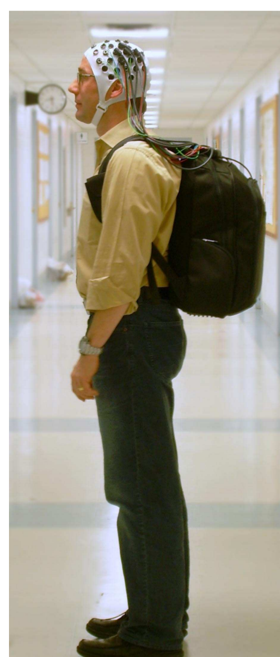
Figure 2. Picture of the instrument. Shown is version with 2 sources, 4 detectors, and 4 trigger connectors for experiment synchronization.
