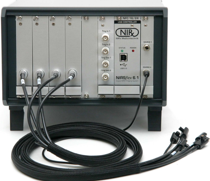
Figure 2. Picture of the instrument. Shown is version with 2 sources, 4 detectors, and 4 trigger connectors for experiment synchronization.
