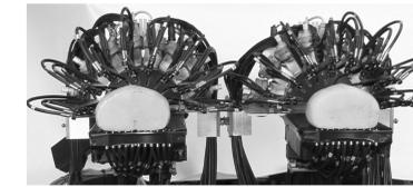
**Figure 1.** Photographs of the simultaneous dual-breast measuring heads, with phantoms in place, for the 1<sup>st</sup>-generation (top) and 2<sup>nd</sup>-generation (bottom) imagers.
