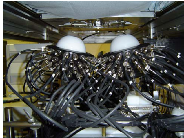
Figure 8. Photograph of measuring head used for simultaneous dual-breast measurements. Thirty-one source-detector fibers are distributed over the surface of each breast.
