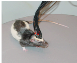
The dental cement used to anchor the implanted side of the connector on the skull is visible as a white band. The weight of the fiber optic bundles is supported by an elastic band, permitting the rat to move freely. With this arrangement, hungry rats will walk around the recording chamber for periods of 15 min or more.
