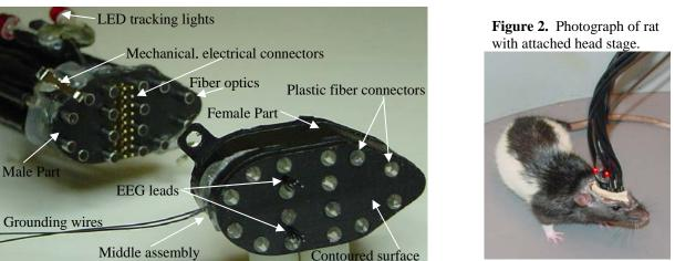
Figure 1. Optical-EEG Head Stage
