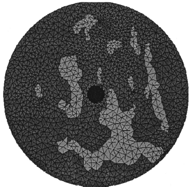
Fig. 1. Medium used in simulation experiments. This finite element mesh was derived from a coronal section of a MR mammogram, following segmentation into three tissue types.
