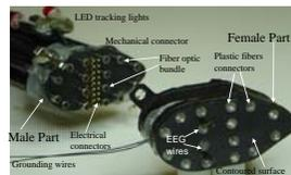
**Figure 2.** Manufactured and assembled headstage.
