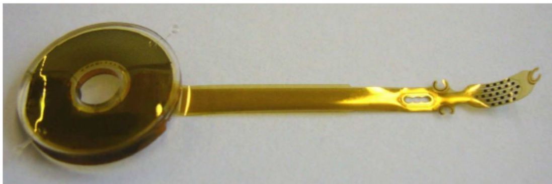
Encapsulated implant with folded microcoil
