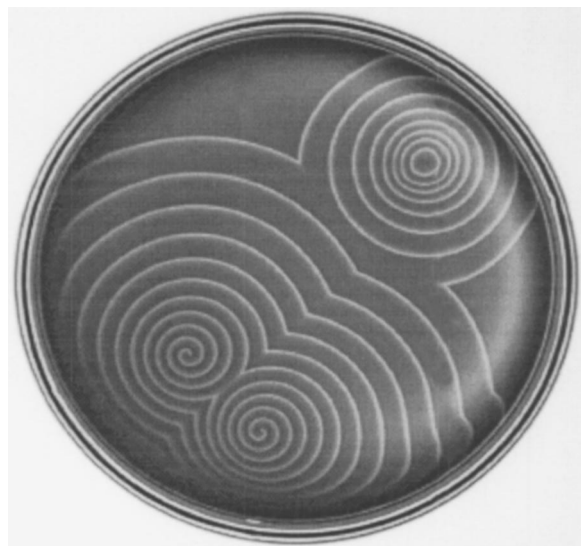
FIG. 1. Picture of chemical waves in the Belousov–Zhabotinsky reaction in a Petri dish. A circular pattern and a counter-rotating spiral pair are visible as bright structures in the dark reaction solution.
